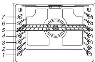
The oven has seven positions for a flat rack, as shown in the previous illustration and the following table.
