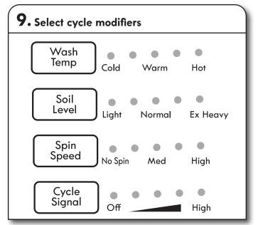
Once you select a cycle, the default modifiers or the previous set modifiers for that cycle will be lit. Touch the cycle settings buttons to change the Wash Temp, Soil Level, and Spin Speed, if desired. Not all settings are available with all cycles.
