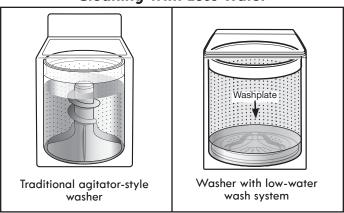
A striking difference in your new washer is the low-water washplate wash system. The washer automatically adjusts the water level to the load size—no water level selector is needed.
