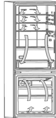
Do not block any of these vents with food packages. If the vents are blocked, airflow will be restricted and temperature and moisture problems may occur.
