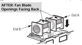
CAUTION: Do not pull or stretch the blower unit wiring. Make sure the wires are not pinched, and that they are properly secured. NOTE: The blower unit exhaust openings should match exhaust openings on rear of microwave oven.
