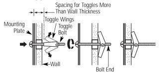
**3** Place the mounting plate against the wall and insert the toggle wings into the holes in the wall to mount the plate.
