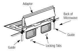
Push in securely until it is in the lower locking tabs. Take care to assure that the damper hinge is installed so that it is at the top and that the damper swings freely.
