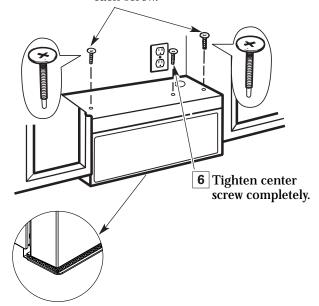
7 Tighten the outer two screws to the top of the microwave oven. (While tightening screws, hold the microwave oven in place against the wall and the top cabinet.)
