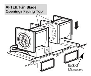
**CAUTION:** Do not pull or stretch the blower unit wiring. Make sure the wires are not pinched, and that they are properly secured.
