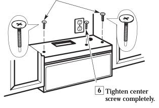
7 Tighten the outer two screws to the top of the microwave oven. (While tightening screws, hold the microwave oven in place against the wall and the top cabinet.)
