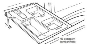
Do not overfill; adding too much detergent may cause detergent to be dispensed into the washer too early.
