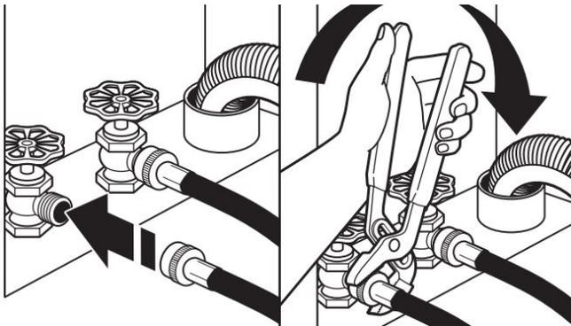
**IMPORTANT:** Do not overtighten or use tape or sealants on valve when attaching to faucets or washer. Damage can result.
