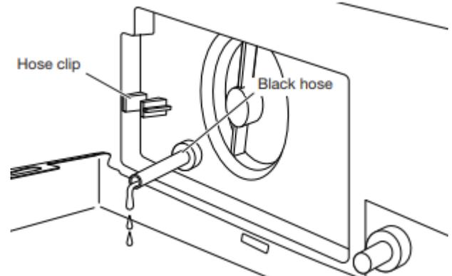
3. Lay a cotton cloth beneath the drain pump filter to absorb any water still in it. Then remove the drain pump filter by turning it counterclockwise.
