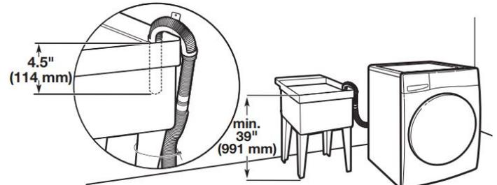
Minimum capacity: 20 gal. (76 L). Top of laundry tub must be at least 39" (991 mm) from the floor; install no higher than 96" (2.4 m) from bottom of washer.
