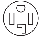
4-wire receptacle (14-30R)
