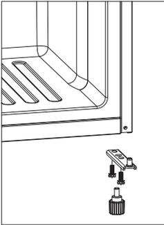
3. Remove the screws holding the bottom hinge with 10mm socket.
