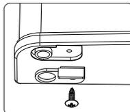
7. Insert left side doorstoppers (provided in your packing) on the left side bottom hole of the refrigerator door and on the left side bottom hole of the freezer door. Fasten with screws provided.
