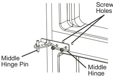
4. Align the holes in the bottom hinge to the corresponding holes on the opposite side of the cabinet. Insert and tighten the screws. Reinstall both front feet.
