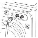
tighten another 2/3 turn with pliers. Do not crossthread or overtighten these connections.
