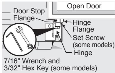
5. Reinstall set screw, locking the door height.
