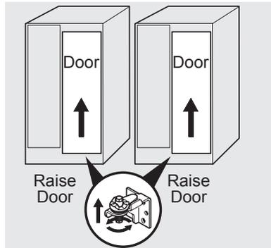
4. After leveling, verify door stop contacts lower hinge and top of door does not contact upper hinge through full movement of door (from fully closed to fully open).
