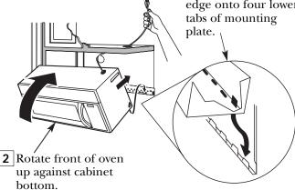
3 Insert a self-aligning screw through top center cabinet hole. Temporarily secure the oven by turning the screw at least **two full turns** after the threads have engaged. (It will be completely tightened later.) Be sure to keep power cord tight. Be careful not to pinch the cord, especially when mounting flush to bottom of cabinet.
