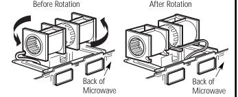
**5** Gently remove the wires from the grooves. Reroute the wires through grooves on other side of the blower unit.
