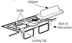
Push in securely until it is in the locking tabs. Take care to assure that the damper hinge is installed so that the damper swings freely.
