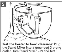
the Stand Mixer into a grounded 3 prong outlet. Turn Stand Mixer ON and test each speed, making sure the beater does not touch the bowl during operation. If the beater is too far away from the bottom or is hitting the bowl, proceed to next step to make adjustments.
