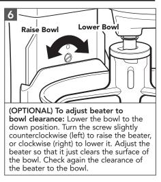
**IMPORTANT:** When properly adjusted, the flat beater will not strike on the bottom or sides of the bowl. If the flat beater or the wire whip is so close that it strikes the bottom of the bowl, coating may wear off the beater or wires on the whip may wear.
