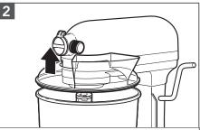
**Remove Pouring shield:** Lift the front of the pouring shield\* clear of the rim of the bowl. Pull away from the Stand Mixer.
