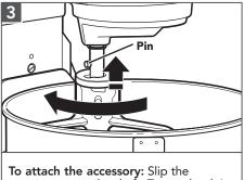
To attach the accessory: Slip the accessory onto the shaft. Turn to hook it over the pin on the shaft.
