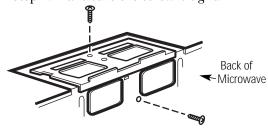
Attach the exhaust adaptor to the top of the blower plate by sliding it into the guides of the blower plate.
