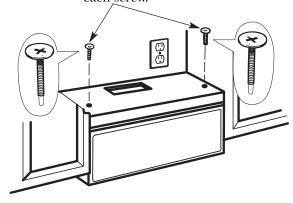
Tighten the outer two screws to the top of the microwave oven. (While tightening screws, hold the microwave oven in place against the wall and the top cabinet.)
