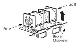
Roll the blower unit 90° so that fan blade openings are facing out the top of the microwave.
