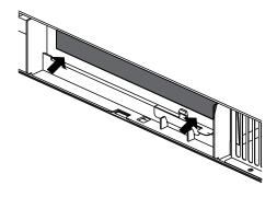
A 5.6 Reinstall the vent by sliding the bottom of the vent into place. Push the vent top into position and slide right into place. Replace the two vent mounting screws located on top of the microwave using a #1 Phillips screwdriver.
