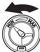
Counterclockwise to reduce foaming
