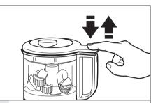
Press rapidly up and down on the handle PULSE/ON button to get your ingredients moving in the work bowl.
