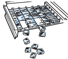
**NOTE:** As the room and water temperatures vary, so will the amount of ice produced and stored. This means that higher operating temperatures will result in reduced ice production.
