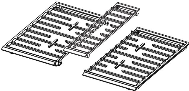
To install the grates, place the grate embossed "Left" on the left side of the cooktop. Place the grate embossed "Right" on the right side of the cooktop. Place the middle grate last, as shown in the previous illustration.
