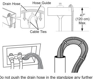
Do not push the drain hose in the standpipe any further than 4" (10 cm). Pushing the drain hose further in the standpipe can cause leaking.
