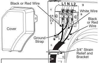
3 #10 AWG minimum copper conductors or 120/240V 30A power supply cord kit marked for use with dryers and provided with closed loop or spade terminals with upturned ends (not supplied).
