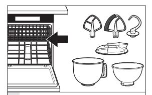
Bowl, pouring shield\*, stainless steel wire whip\*, stainless steel flat beater\*, stainless steel dough hook\*, white flat beater\*, Flex Edge beater\*, and white dough hook\* may be washed in a dishwasher. Or, clean them thoroughly in hot sudsy water and rinse completely before drying. Do not store beaters on shaft.
