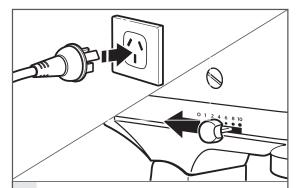
Plug the Stand Mixer into a proper electrical outlet. Always set speed control lever on lowest speed to start, then gradually increase speed to avoid splashing ingredients. See the "Speed control guide" chart.
