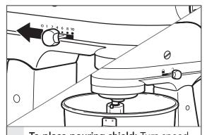
To place pouring shield: Turn speed control to "0". Unplug Stand Mixer.
