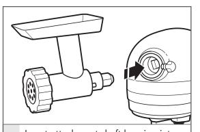
Insert attachment shaft housing into attachment hub, making certain that attachment power shaft fits into square attachment hub socket. It may be necessary to rotate attachment back and forth. When attachment is in proper position, the pin on the attachment will fit into the notch on the hub rim.
