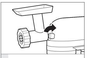
Tighten attachment knob by turning clockwise until attachment is completely secured to Stand Mixer.
