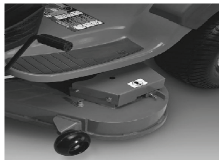
Fabricated Deck Shell Example Below
