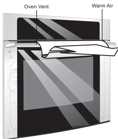
Figure 1: Oven vent locations
