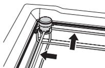
2. As the divider has the width and length bars, push the lower part of each bar inward to unlock. See the pictures for details.
