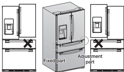
The left door is fixed. To make minor adjustments between doors, adjust only the right door.
