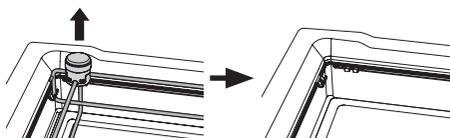
4. Turn over the drawer to remove the metal cooling plate.
