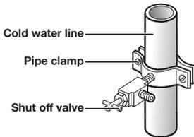
3. Connect the water line installation kit to the shut off valve.
