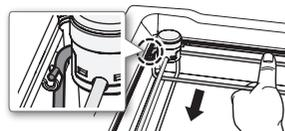
3. Hold the divider and pull up to remove.
