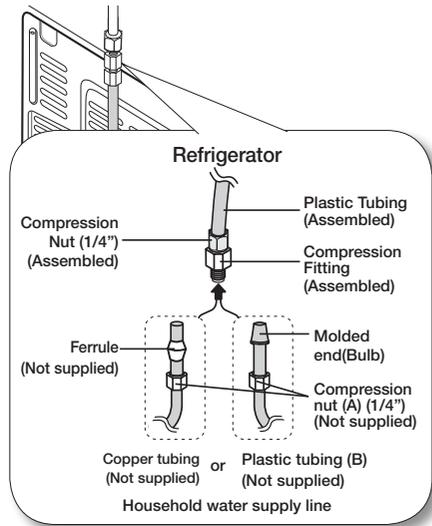
1. Connect the household water line to the assembled compression fitting.
