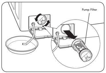
Twist the pump filter counterclockwise to remove. Remove any lint and foreign objects from the pump filter. Insert pump filter back into opening and twist clockwise to secure. Insert the plug in the drain hose and reclip the hose. Be sure to close the drain pump filter access panel.
