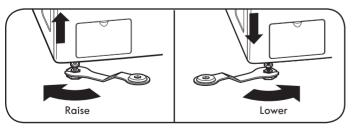
2. Loosen the locknuts on all four leveling feet with the wrench until you can adjust the feet (wrench appearance may vary). Use the wrench to turn the feet clockwise to raise the washer, and counterclockwise to lower the washer. Using a level, adjust the feet until the washer is level from side to side and front to back. Make sure that all four feet are in firm contact with the floor.
