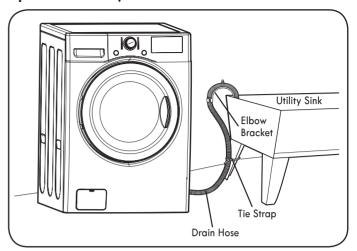
Install the elbow bracket near the end of the drain hose. Hang the end of the drain hose over the side of the utility sink. Use a tie strap to secure the drain hose in place.
