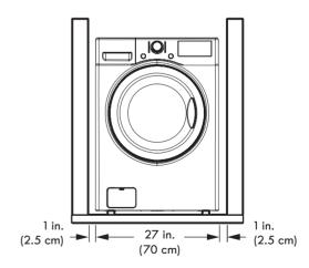
**NOTE:** The floor must be strong and rigid enough to support the weight of the washer, when fully loaded, without flexing or bouncing. If your floor has too much flex, reinforce it to make it more rigid.
