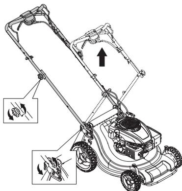
2. Tighten the lower handlebar knobs.
