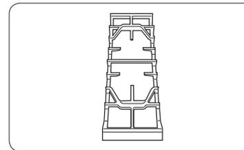
Samsung gas ranges come with a center burner grate. This grate fits over the center oval burner. The center burner grate should not be used over any other burners and no other center stovetop grates should be used with this range.
