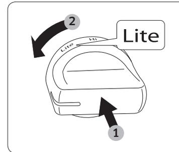
1. Push in the control knob, and then turn it to the Lite position. You will hear a "clicking" sound indicating the electronic ignition system is working properly.
