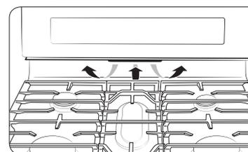
The oven vent is located under the oven Control panel. Proper air circulation prevents oven burner combustion problems and ensures good performance.
