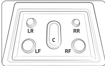
Each burner has a corresponding knob that lets you to set the flame level from LO to HI. In addition, each burner knob has a Lite setting. Turning a knob to Lite ignites the corresponding burner. The burner indicators are located above each knob and show which burner the knob controls. Each burner is designed for specific cooking purposes. See the table below.
