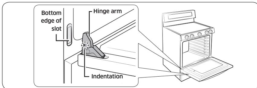
3. Open the door fully. If the door will not open fully, the indentation is not inserted correctly in the bottom edge of the slot.
