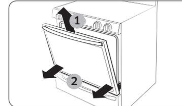
4. Close the door to 5 degrees from vertical. This is the removal position.
