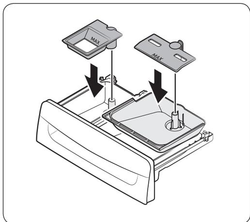
3. Remove the inserts from the compartments. Rinse the inserts and the drawer in warm water and clean with a soft brush.
