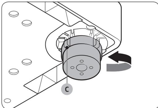
1. Slightly lift the washer, and then turn the **leveling feet (C)** counterclockwise to separate it from the washer.
