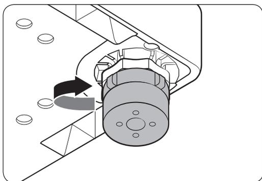
4. Put the leveling feet back to the washer, and then turn it clockwise until it is fully retracted.
