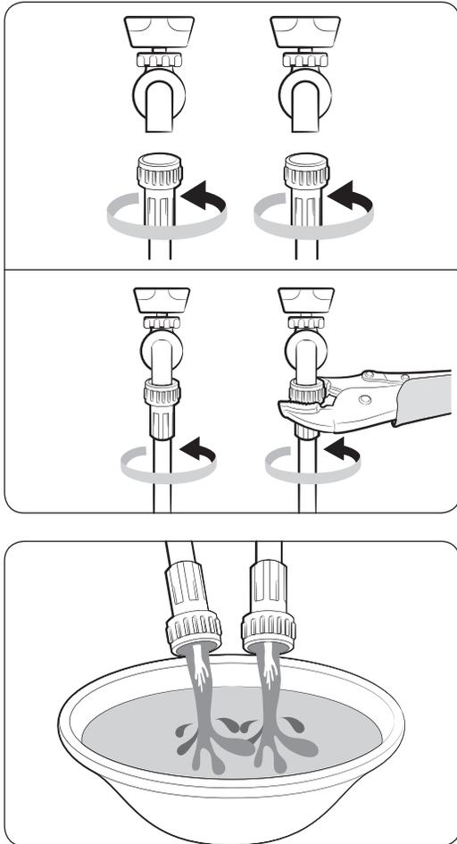
1. Attach the water hoses to the hot and cold water taps, and then hand tighten the water hose fittings until they are tight. Then, use pliers to tighten the fittings by an additional two-thirds of a turn. To avoid damaging the fittings, do not overtighten them.
