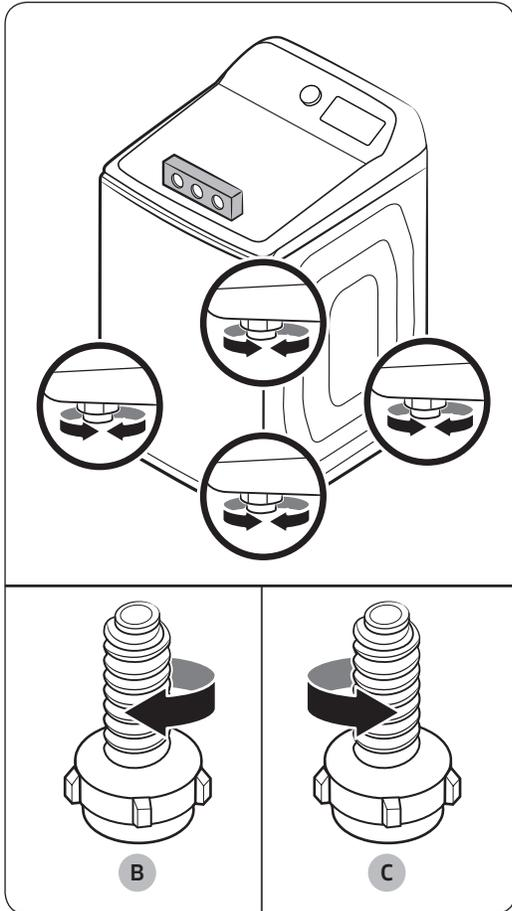
4. If the washer is not level, turn the appropriate leveling feet **clockwise (B)** to lower the washer, or **counterclockwise (C)** to raise the washer so that it is level.
