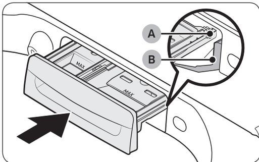
5. Return the inserts to the proper compartments. Replace the drawer by placing the **drawer rail (A)** on the **compartment rail (B)** while tilting the drawer downward.
