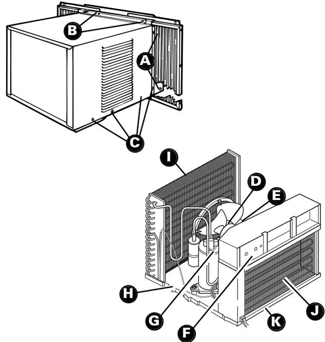
8. Carefully clean and hose out base (H), condenser coil (I), evaporator coil (J), and condensate pan (K). Clean at least once a year or more often if the condenser and evaporator coils and pan collect dirt, sand, leaves, insects, or algae. Also, clean if you detect an odor coming from the air conditioner.
