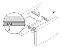
**5** Grip both sides of the drawer and pull it up to remove it from the rails.
