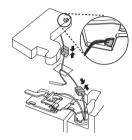
4 Place the hinge cover in place. Insert and tighten the cover screw.
