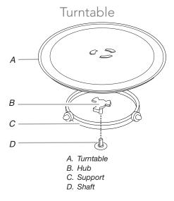
The turntable can rotate in either direction to help cook food more evenly. For best cooking results, do not operate the microwave oven without having the turntable in place. See the "Assistance or Service" section to reorder any of the parts.
