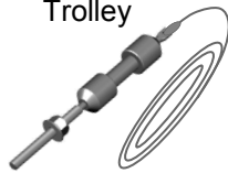
Trolley Shaft and Cable
