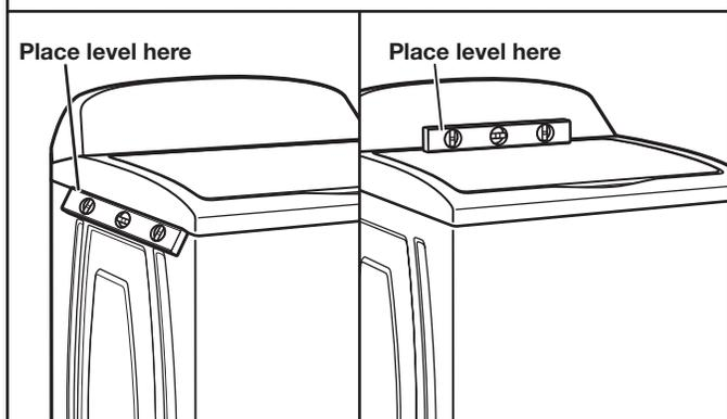
Move the washer to its final location. Place a level on top edges of washer. Use side seam as a guide to check levelness of sides. Check levelness of front using lid, as shown. Rock washer back and forth to make sure all four feet make solid contact with floor. If washer is level, skip to step 15.
