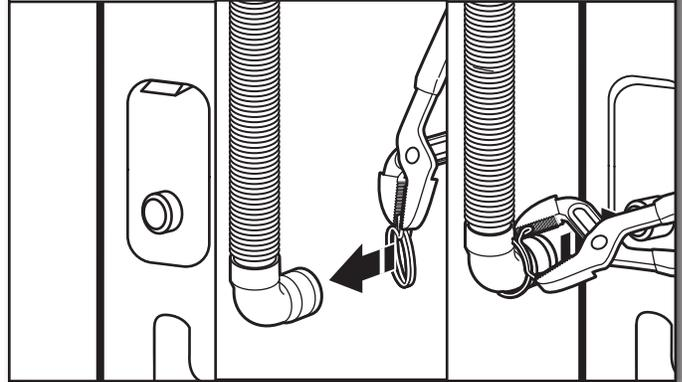
If clamp is not already in place on elbow end of drain hose, slide it over end as shown. Squeeze clamp with pliers and slide black elbow end of drain hose onto black drain port and secure with clamp.
