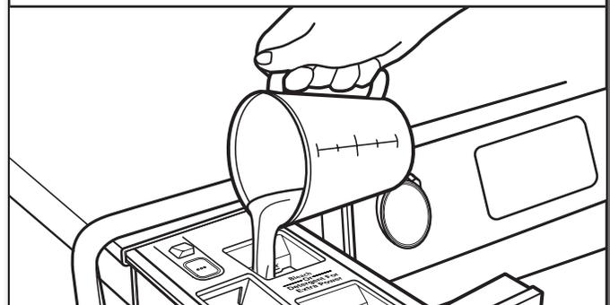
Add liquid chlorine bleach to the bleach compartment. Do not overfill, dilute, or use more than manufacturer's recommendation for dosing. Do not use color-safe bleach or Oxi in the same cycle with liquid chlorine bleach.
