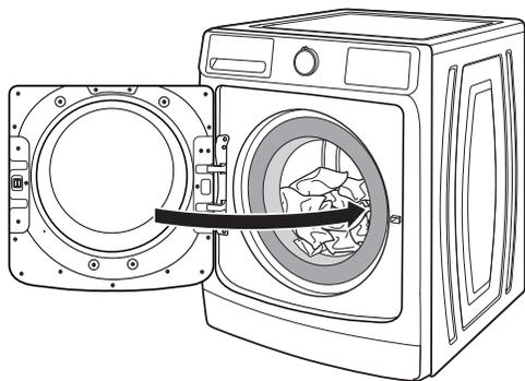
Place a load of sorted items loosely in the washer. Items need to move freely for best cleaning and to reduce wrinkling and tangling. Close the washer door by pushing it firmly until the latch clicks.
