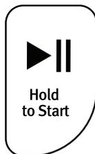
Touch and hold START to start the wash cycle. To pause a cycle in progress, touch START once, then touch and hold again to continue the cycle. To cancel a cycle, touch POWER.
