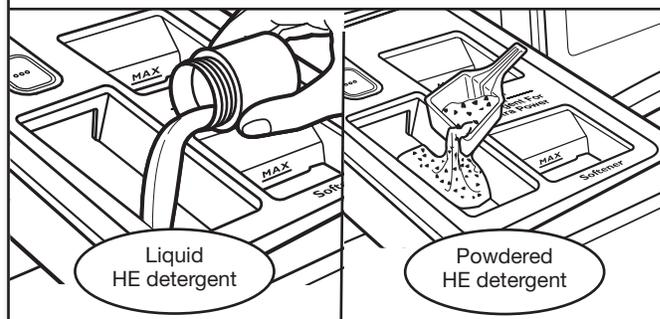
Adjust the selector, based on type of HE detergent used (either liquid or powdered). See “Using the Dispenser Drawer” section on how to use the dispenser.
