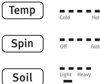
The display will show the default settings for the selected cycle. To adjust a setting, touch its name – Temp, Spin or Soil. Adjusting settings will change the Estimated Cycle Time. Tightly packing the load, unbalanced loads, or excessive suds may also cause the washer to increase the cycle time.
