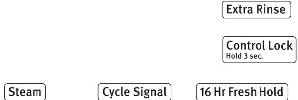
To add an option to the cycle, touch its name – Fresh Hold, Steam, Extra Rinse, Cycle Signal, or Control Lock. To remove an option from the selected cycle, touch the option again.
