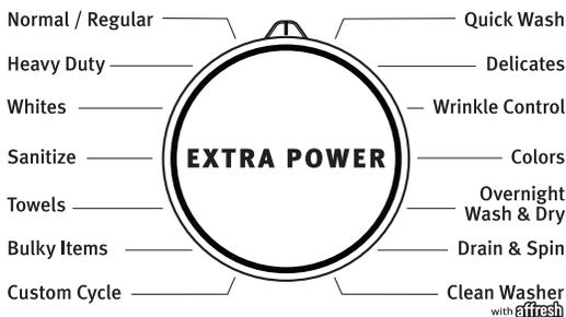
Turn cycle knob to select your wash cycle. See “Cycle Guide” for details on cycle features. Press the knob for enabling the Extra Power option.
