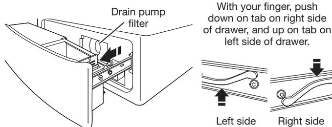
2. Place a broad, flat container beneath the drain pump filter to collect the drain water. Release the black hose from the hose clip, remove the plug, and drain the hose into the container. Empty the container. Repeat this procedure if necessary until all the water has drained. Make sure that the black hose is completely dry, replace the plug, and secure the hose in the clip.
