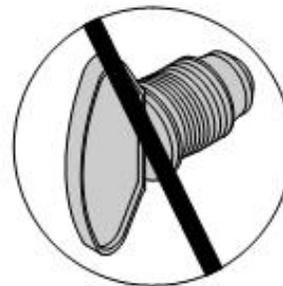
**Do not insert a POL transport plug (plastic part with external threads) into the type 1 valve outlet. It will defeat the Safety Relief Valve feature.**
