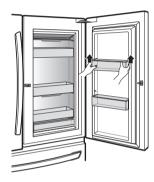
To replace the door bins, slide the door bin in above the desired support and push down until it snaps into place.
