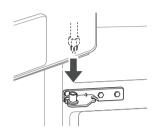
2 Fit the hinge (1) over the hinge lever latch and slot it into place. Rotate the lever clockwise (2) and fasten the hinge.
