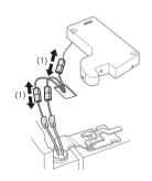
Rotate the hinge lever (1) clockwise. Lift the top hinge (2) free of the hinge lever latch.
