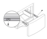
Grip both sides of the drawer and pull it up to remove it from the rails.
