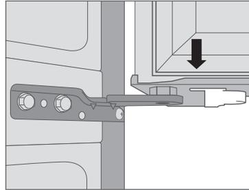
2. Fit the top hinge over the mounting holes and align to proper position before tightening. Turn top hinge fastener clockwise to secure the hinge.
