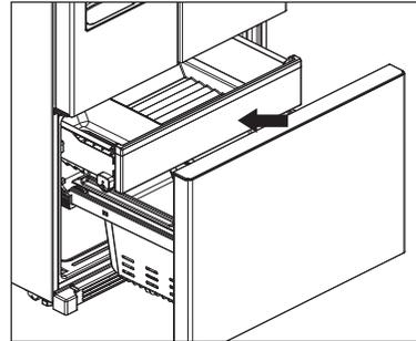
2. Fully push in and close freezer drawer to engage rails with rail support locking tab, applying a bit of pressure after the door is closed to seat the tabs to the rail.
