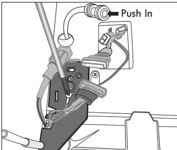
3. Using a large phillips screwdriver, turn top hinge fastener counterclockwise to remove the top hinge plate.
