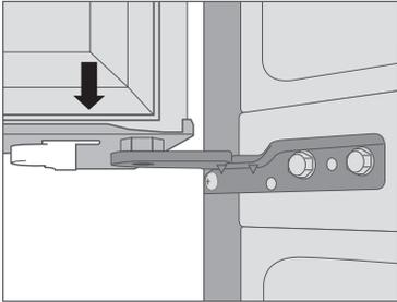
2. Fit the top hinge over the mounting holes and align to proper position before tightening. Turn top hinge fastener clockwise to secure the hinge. Securely reconnect the grounding wires, wire harnesses and water tube. Simply push the water tube back into the collar to connect.
