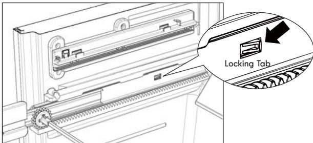
4. Pull exterior freezer drawer to fully disengage the rail assembly from the unit. Use 2 people for this task as the door is heavy and awkward to handle.
