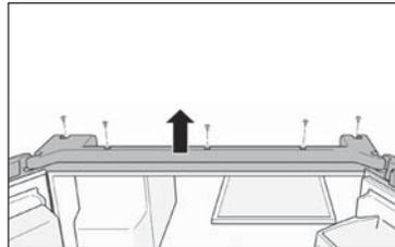
2. Using a large phillips screwdriver, turn top hinge fastener counterclockwise to remove the top hinge plate.
