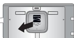
1. Insert fingertips beneath base of filter cover and pull toward you to remove.
