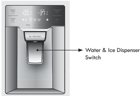
When Ice Select button is pressed once, cubed ice will dispense. Press Ice Select button a second time to dispense crushed ice.
