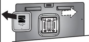
2. Turn cover over. Slide filter to right to remove. Slide new filter to left to insert.
