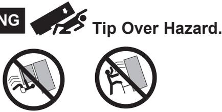
Built-in style models (model PYE, GYE, GYS, PWE, and ZWE) are top heavy, especially with any doors open. These models must be secured with the anti-tip floor bracket to prevent tipping forward, which could result in death or serious injury. Read and follow the entire installation instructions for installing the anti-tip floor bracket packed with your refrigerator.
