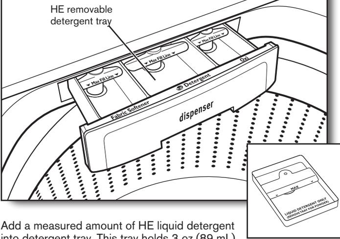
Add a measured amount of HE liquid detergent into detergent tray. This tray holds 3 oz (89 mL). If adding powder HE detergent remove inside tray. Do not overfill tray – adding too much detergent may cause detergent to be dispensed into the washer too early.
