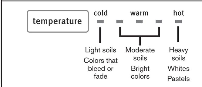
Once you select a cycle, select the wash temperature by touching the Temperature button to the desired setting. Even for cold wash settings, some warm water may be added to the washer to maintain a minimum temperature.
