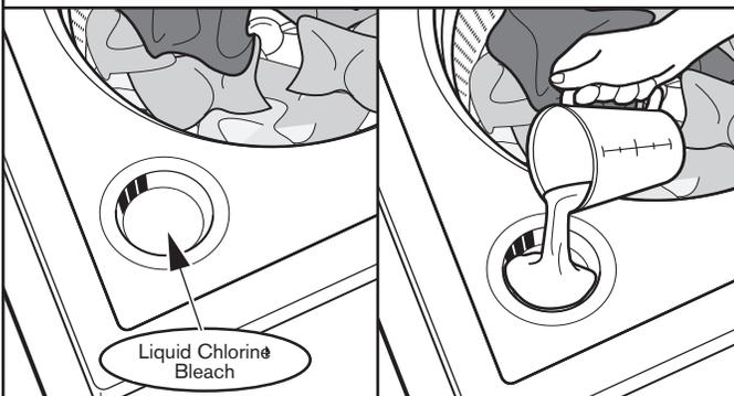
Do not overfill, dilute, or use more than 1 cup (236 mL). Do not use color-safe bleach or Oxi products in the same cycle with liquid chlorine bleach.
