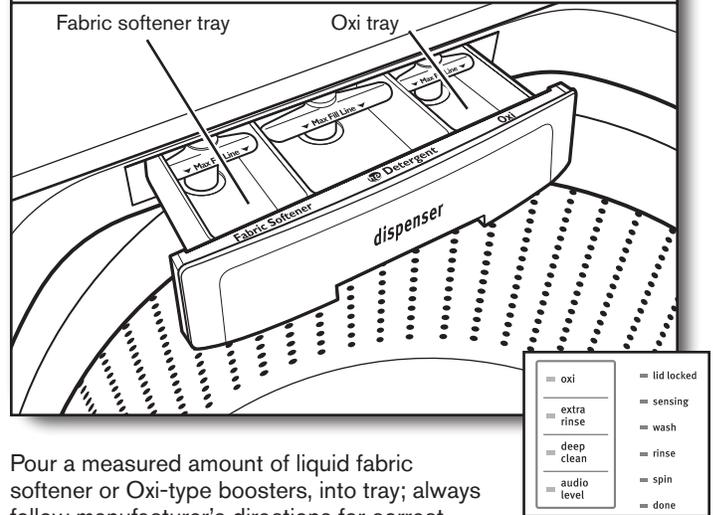
Pour a measured amount of liquid fabric softener or Oxi-type boosters, into tray; always follow manufacturer’s directions for correct amount of fabric softener or Oxi based on your load size. Close dispenser drawer, and then select Oxi option. Oxi is added during main wash and Fabric Softener is added during rinse.
