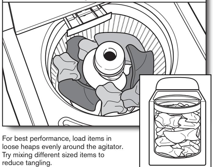
For best performance, load items in loose heaps evenly around the agitator. Try mixing different sized items to reduce tangling.
