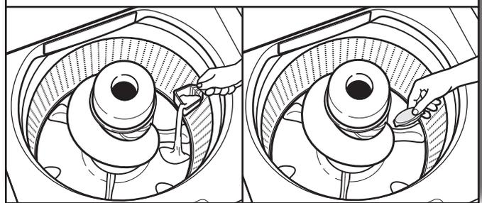
Single-dose laundry packet, color-safe bleach, or fabric softener crystals can be added to the basket prior to adding laundry.
