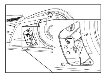
When the Drive Belt (59) is tight, tighten the Idler Pivot Screw (76). Then, reattach Access Cover (29) and plug in the power adapter.
