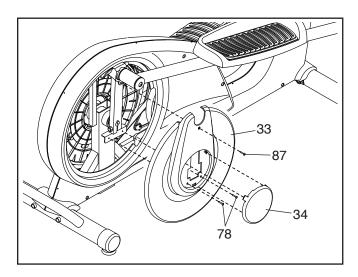
Then, remove the M8 x 12mm Screw (87) and the two M4 x 16mm Screws (78) from the right Disc (33), and then remove the right Disc.
