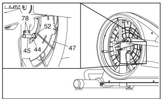
Next, rotate the Pulley (47) until a Magnet (52) is aligned with the Reed Switch (44). Slide the Reed Switch slightly toward or away from the Magnet. Then, retighten the M4 x 16mm Screws (78).
