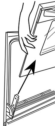
**NOTE:**The oven door is very heavy. Be sure you have a firm grip before lifting the oven door off the hinges. Use caution once the door is removed. Do not lay the door on its handle. This could cause dents or scratches
