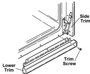
**CAUTION:** Be sure you do not tip the oven forward during installation or you may bend the Bottom Trim. The Bottom Trim provides an opening for cooling air to enter the cabinet. This opening should never be blocked.
