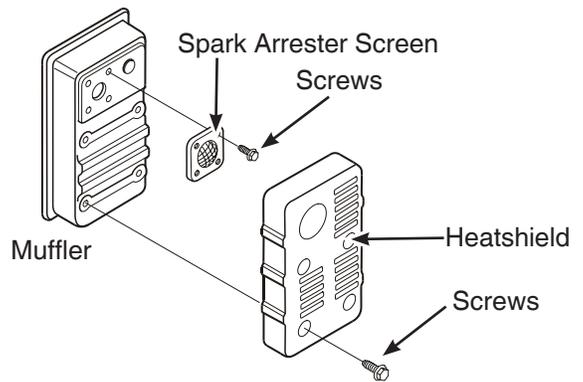
2. Remove four screws that attach spark arrester screen.
