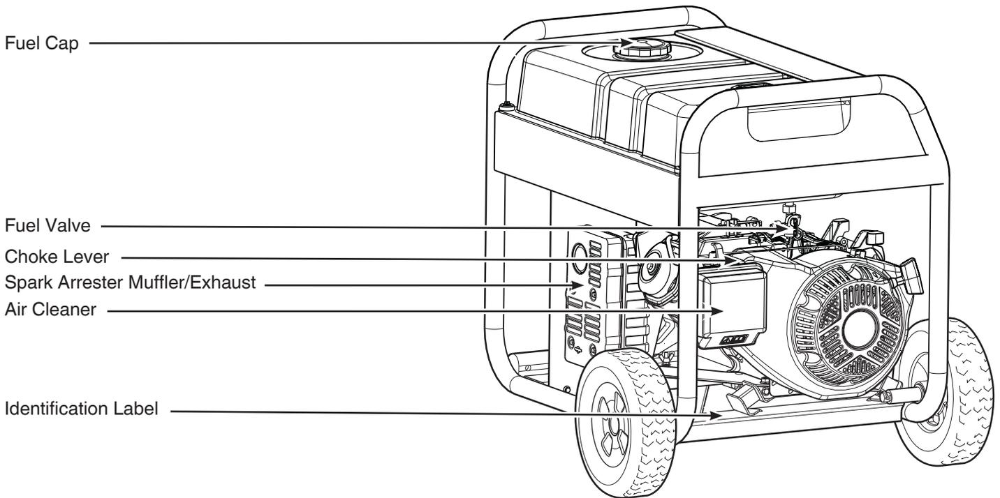
Air Cleaner — Filters engine intake air.
