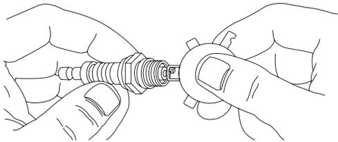
5. Install spark plug and tighten firmly.
