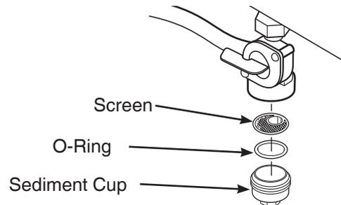
3. Wash sediment cup, o-ring, and screen in a nonflammable solvent. Dry them thoroughly.
