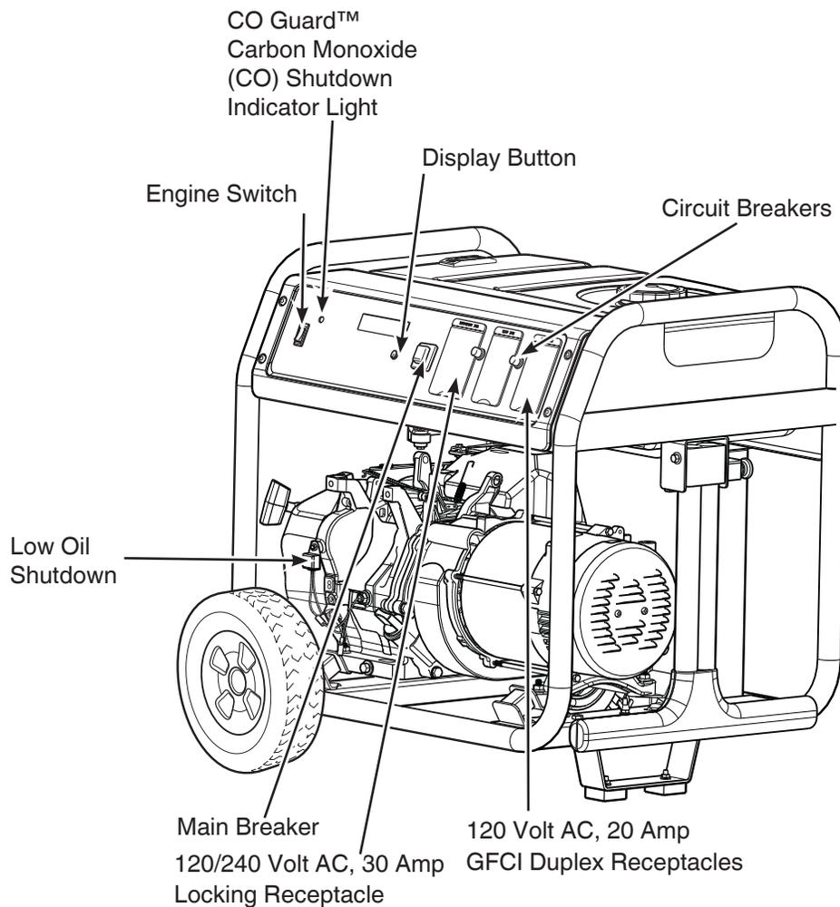
120 Volt AC, 20 Amp, GFCI Duplex Receptacles — Used to supply 120 Volt AC, single phase, 60 Hz power for electrical lighting, appliance, tool and motor loads.
