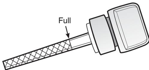
4. If needed, slowly pour oil into oil fill opening to the full mark on dipstick. Do not overfill.
