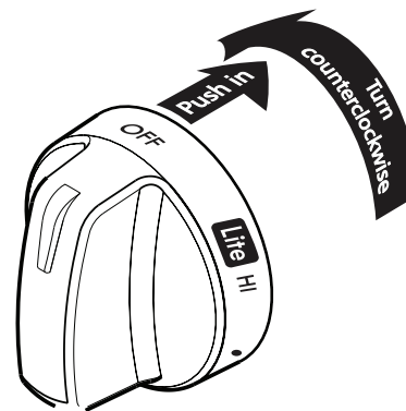
Figure 8: Proper way to set burners
