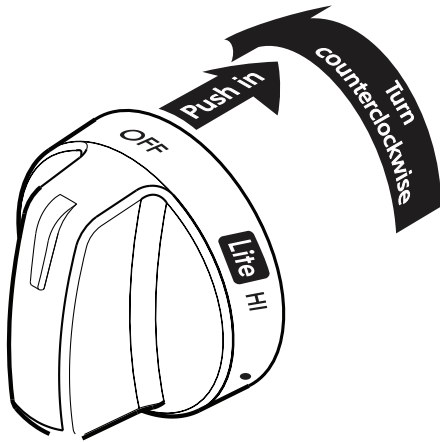
Figure 9: Setting the double ring burner
