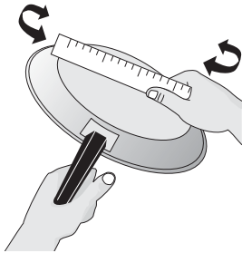
Figure 6: Check for flat bottom cookware
