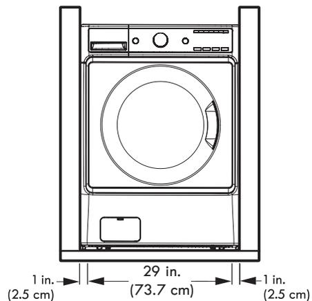
Allow at least 25 13/16 in. (65.5 cm) in front of the washer to open the door.
