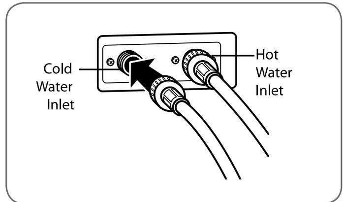
**WARNING:** Do not overtighten the hoses. Overtightening can damage the valves resulting in leaking and property damage.
