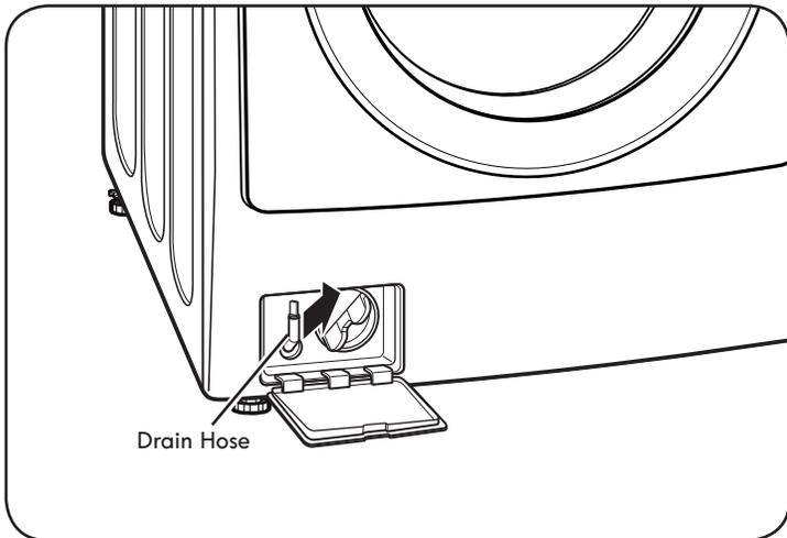
**2** Unclip the drain hose and pull it out. Place the end of the drain hose into a shallow pan or a floor drain. Make sure not to pull the hose out too far, or it may not drain properly.
