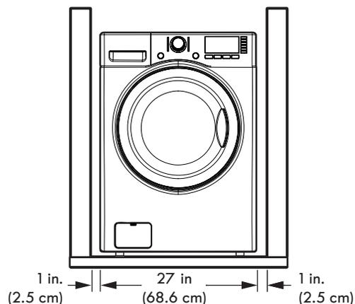
Allow at least 22 1/4 in. (56.6 cm) in front of the washer to open the door.
