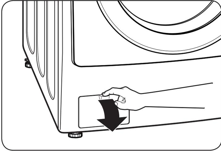
**1** Open the drain pump filter access panel.
