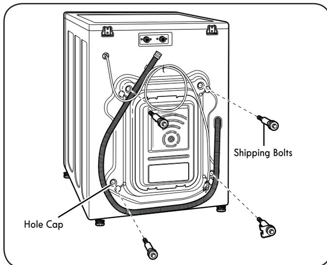
2. Remove the bolt assemblies by wiggling them slightly while pulling.
