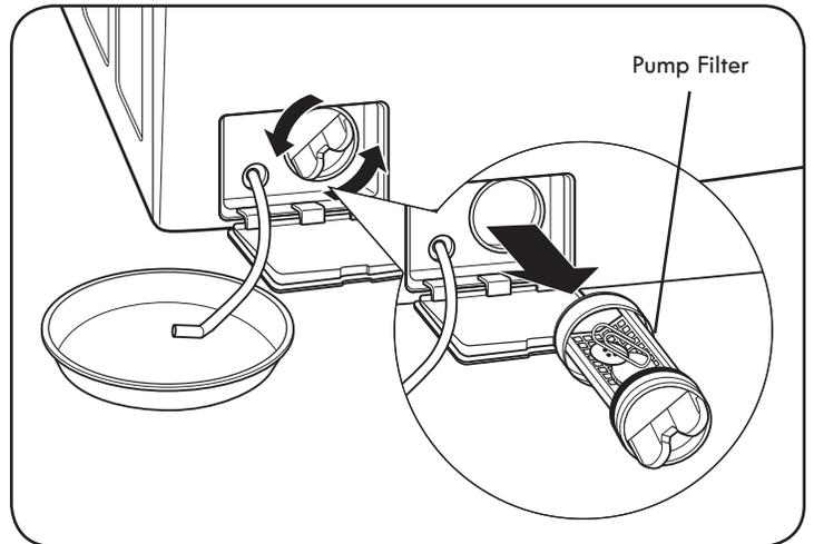
**4** Twist the pump filter counterclockwise to remove. Remove any lint and foreign objects from the pump filter. Insert pump filter back into opening and twist clockwise to secure. Be sure to close the drain pump filter access panel.
