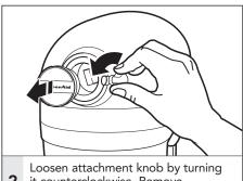
Loosen attachment knob by turning it counterclockwise. Remove attachment hub cover.
