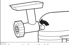
Loosen attachment knob by turning it counterclockwise. Rotate attachment slightly back and forth while pulling out.
