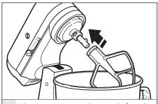
Slip accessory onto beater shaft and press upward as far as possible. Then, turn accessory to the right, hooking accessory over the pin on the shaft.
