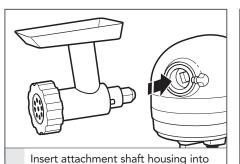
attachment hub, making certain that attachment power shaft fits into square attachment hub socket. It may be necessary to rotate attachment back and forth. When attachment is in proper position, the pin on the attachment will fit into the notch on the hub rim.
