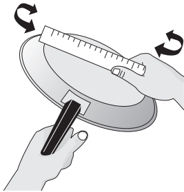
Figure 6: Check for flat bottom cookware
