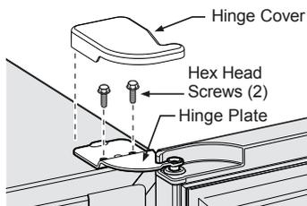
3. Hold the door in place while removing the top hinge from the cabinet.
