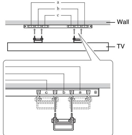
**2** Adjust the angle of the Mounting Hook.
