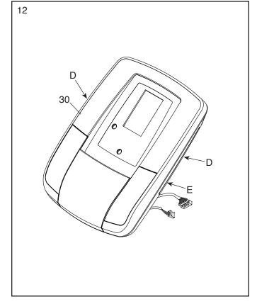
13. Remove and discard the wire tie on the Main Wire (32).
