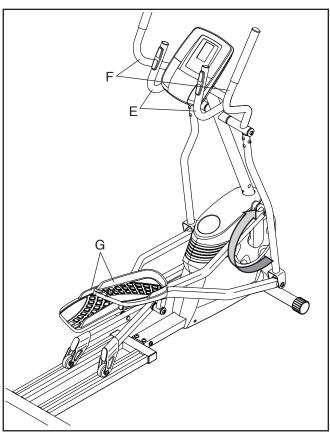
To dismount the elliptical, wait until the pedals (G) come to a complete stop. Note: The elliptical does not have a free wheel; the pedals will continue to move until the flywheel stops. When the pedals are stationary, step off the higher pedal first. Then, step off the lower pedal.
