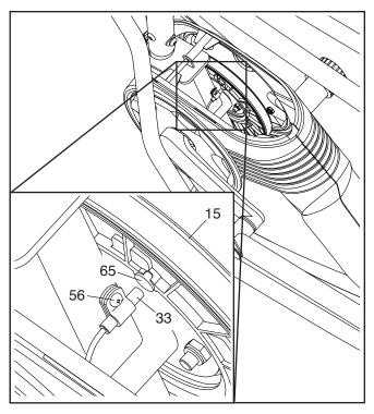
Slightly loosen the indicated M4 x 16mm Screw (56). Slide the Reed Switch (33) slightly closer to or away from the Magnet (65), and then retighten the Screw. Then, rock the Pulley (15) forward and backward just enough that the Magnet passes the Reed Switch repeatedly.
