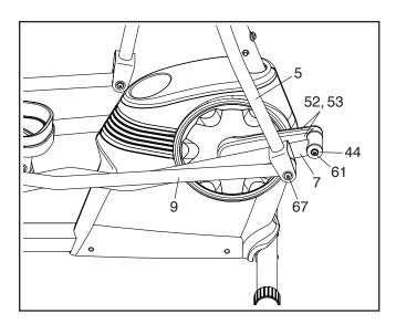
Next, remove the M8 x 20mm Screw (61), the Axle Cover (44), and the M8 Washer (not shown) from the Right Roller Arm (7) and the right Crank Arm (not shown). Gently move the Right Roller Arm out of the way. Then, use a standard screwdriver and gently remove the Outer and Inner Crank Covers (52, 53) from the right Crank Arm.
