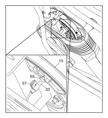
Loosen, but do not remove, the indicated M4 x 12mm Screw (57). Slide the Reed Switch (33) slightly closer to or away from the Magnet (65), and then retighten the Screw. Then, rock the Pulley (15) forward and backward just enough that the Magnet passes the Reed Switch repeatedly.
