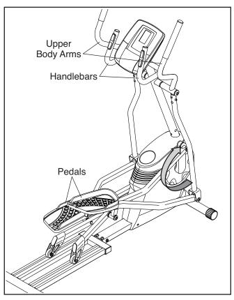
To dismount the elliptical, wait until the pedals come to a complete stop. Note: The elliptical does not have a free wheel; the pedals will continue to move until the flywheel stops. When the pedals are stationary, step off the higher pedal first. Then, step off the lower pedal.
